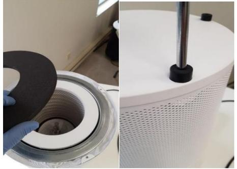
6. INSTALL THE HEPA FILTER. MAKE SURE THE PREFILTER AND THE TREPA ARE NOT COVERING THE BOTTOM BRACKETS. ADD THE UPPER GASKET AND THE BOTTOM COVER AND REPLACE THE 4 SCREWS
