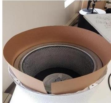
1. INSTALL THE CARBON FILTER. BE CAREFUL NOT TO CATCH THE EDGES OF THE SLIDER. MAKE SURE THE CARBON FILTER IS ALLTHE WAY IN AND SITS ON THE FOAM GASKET
