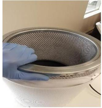
6. REMOVE THE CARBON FILTER BY FIRMLY PULLING IT OUT. THE PREFILTER IS HOLDING ON THE CARBON FILTER SO YOU HAVE TO OSCILATE THE MOVMENTS WITH BOTH HANDS IN ORDER TO RELEASE IT.
